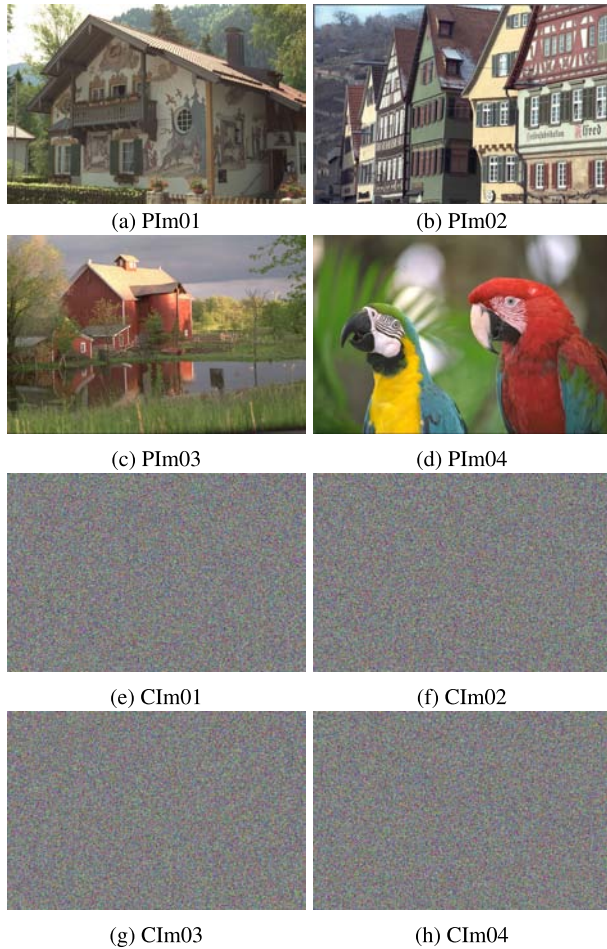
FIGURE 17. Experimental dataset of images, which the first two rows indicate the plain images and it's corresponding ciphered ones are provided in the last two rows.
