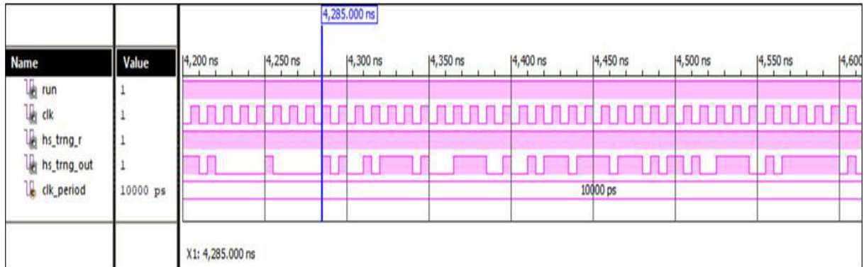
FIGURE 14. The timing diagram results of dual core high speed hybrid TRNG using Ring and Heun algorithm based on the new 5-D hyperchaotic oscillator on FPGA obtained from Xilinx ISE Simulator.
